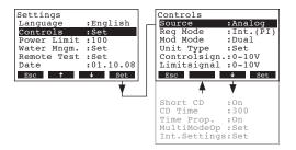
The display with control settings appears. The settings available depend on the selected signal source, the regulation mode and the modulation mode. The display above shows the maximum number of settings available. Please refer to the following chapters for further information on the individual control settings.
