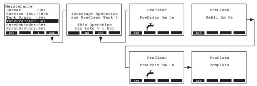
You are asked whether you want to stop operation and drain the tank. Press the **<Yes>** key. The pre-clean functions starts. During the tank pre-clean cycle the display confirms the tank is drained and filled along with the time remaining to complete the procedure.
