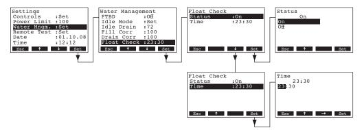
In the upcoming float check submenu select "Status" to activate or deactivate the float check function or select "Time" to set the hours of day at which the float check should be started (format: hh:mm).
