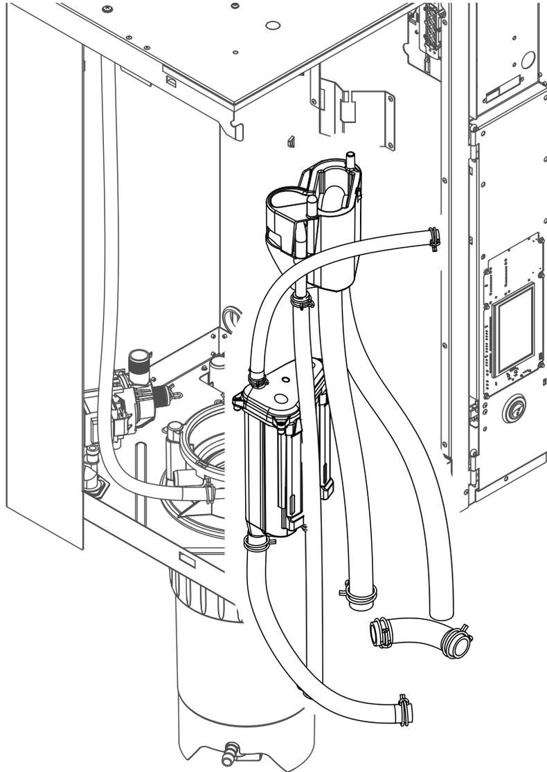
1. Release hose clamps, then disconnect all hoses from the corresponding connectors and remove the hoses.
