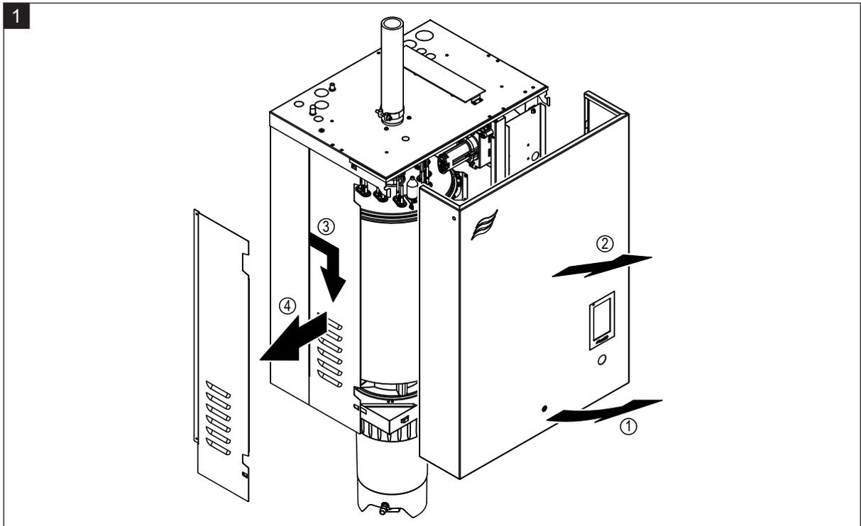
1. Loosen retaining screw on front door or on left front door (for large units) of the unit using a screwdriver, then remove the front door. Pull left side panel to the front and then downwards and remove side panel.
