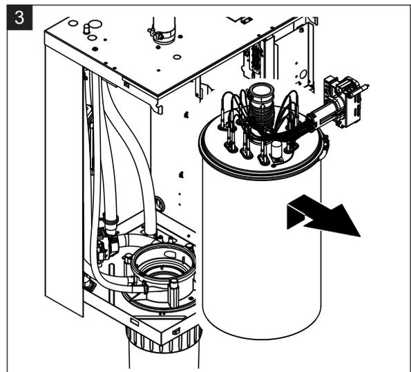
2. Free the upper hose clamp of the steam outlet hose using a screwdriver and pull the hose downwards from the steam connector. Then, loosen the two screws fixing the heating cable plug to the plug socket and remove heating cable plug from the plug socket.
