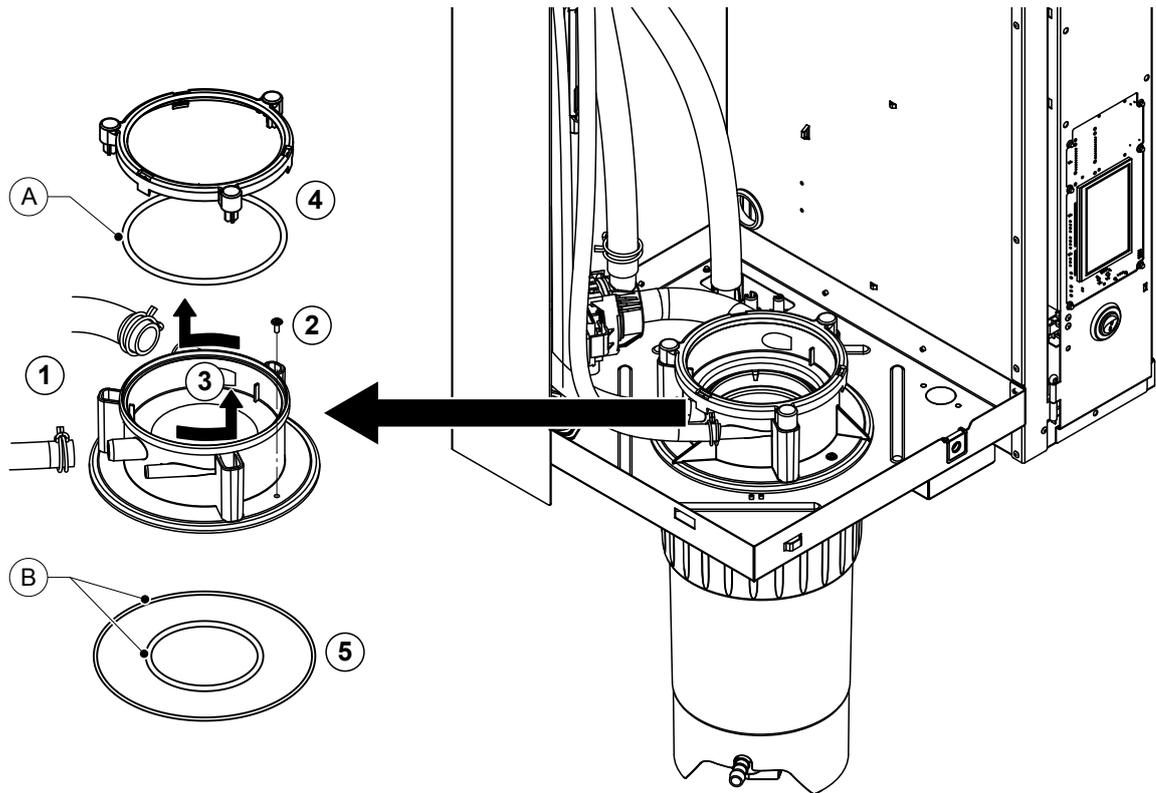
1. Release hose clamps and remove hoses from the connectors.
